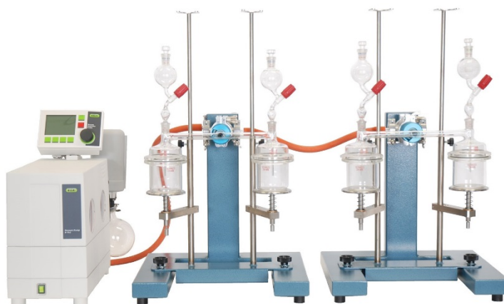
Figure 16: Real density determination apparatus (RDC 152 / 186 / 198)
