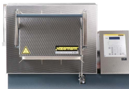
Figure 18: Furnace for Ash Content RDC 169
