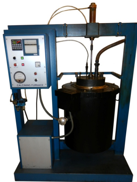
Figure 3: RDC 165 Söderberg baking furnace BF12S
